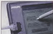
Philips Velo 1: Don't worry about finding a free slot when you want to go online. The Velo 1 has a space-saving built-in software modem. Just plug your phone line into the pop-up jack.
